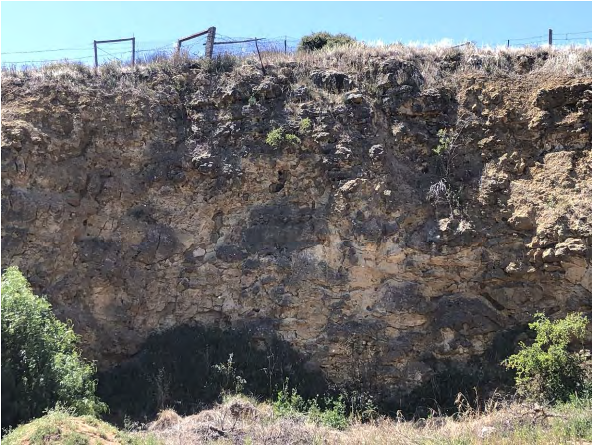
Figure 4: Outcropping Limestone on a Near Vertical Cliff Slope (near BH5, Facing Southwest)
